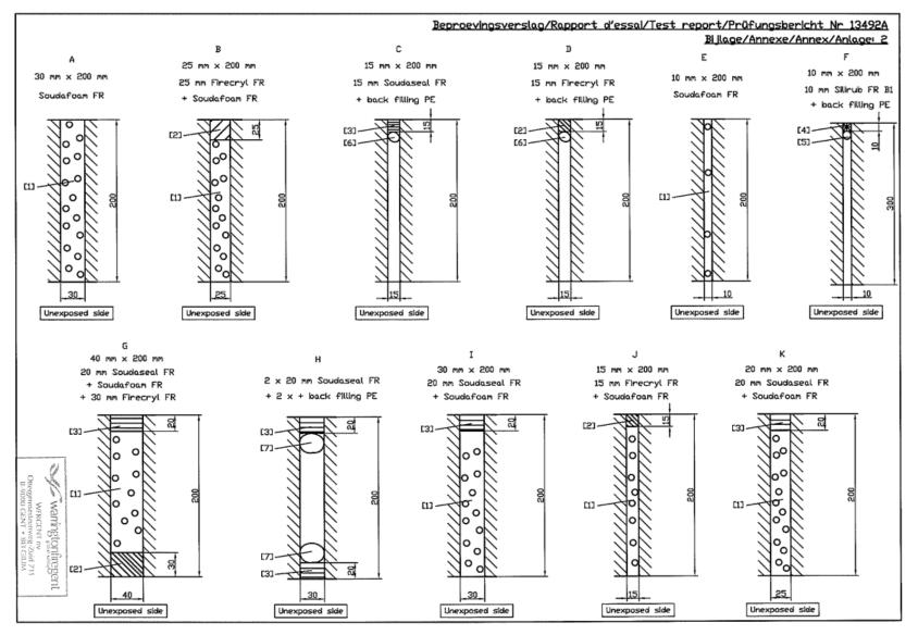
Figure 1 Tested sealant configurations
