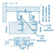
When door thickness is determined use dimensions on chart below for correct positioning of track on head and correct hanger for front and rear doors.
