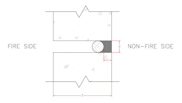
Figure 2 – Typical sealant insulation
