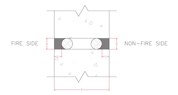
Figure 1 – Typical sealant insulation
