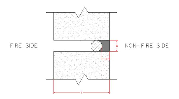
Figure 8 – Typical sealant insulation
