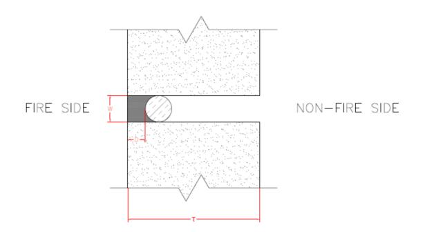
Figure 8 – Typical sealant insulation
