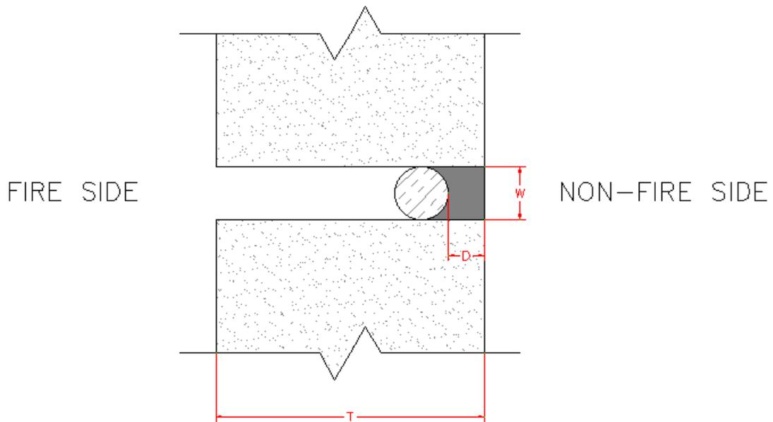
**Figure 8 – Typical sealant insulation**
