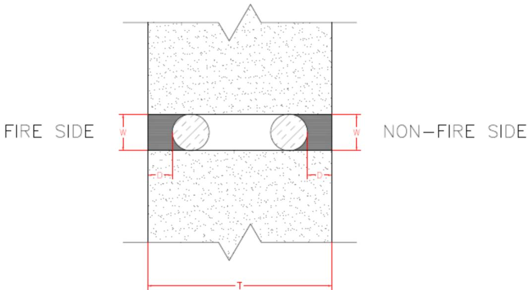
**Figure 7 – Typical sealant insulation**
