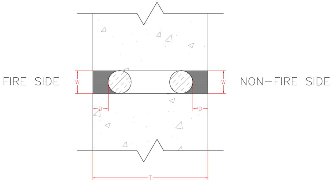
Figure 1 – Typical sealant insulation
