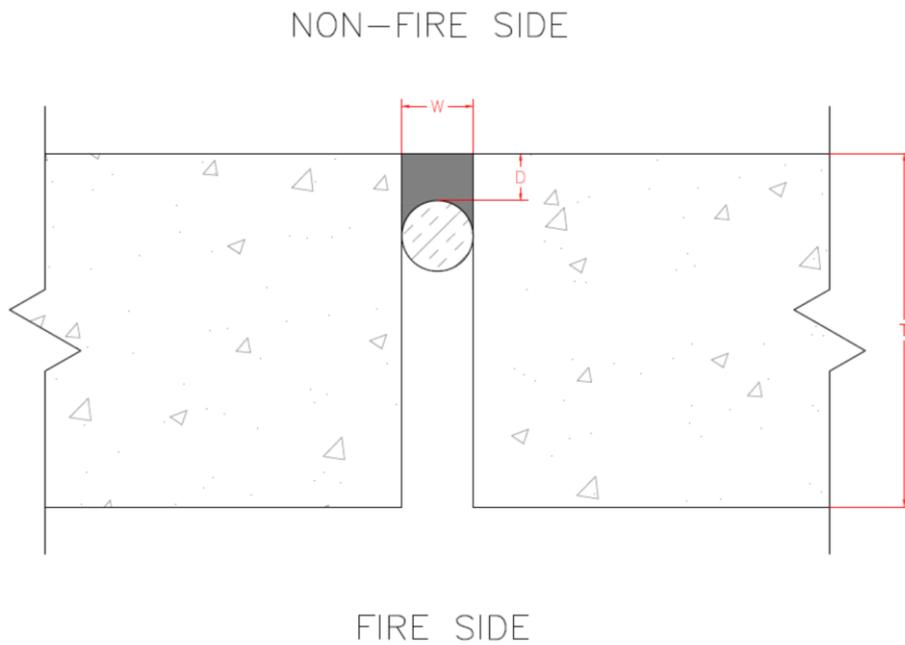
**Figure 4 – Typical sealant insulation**
