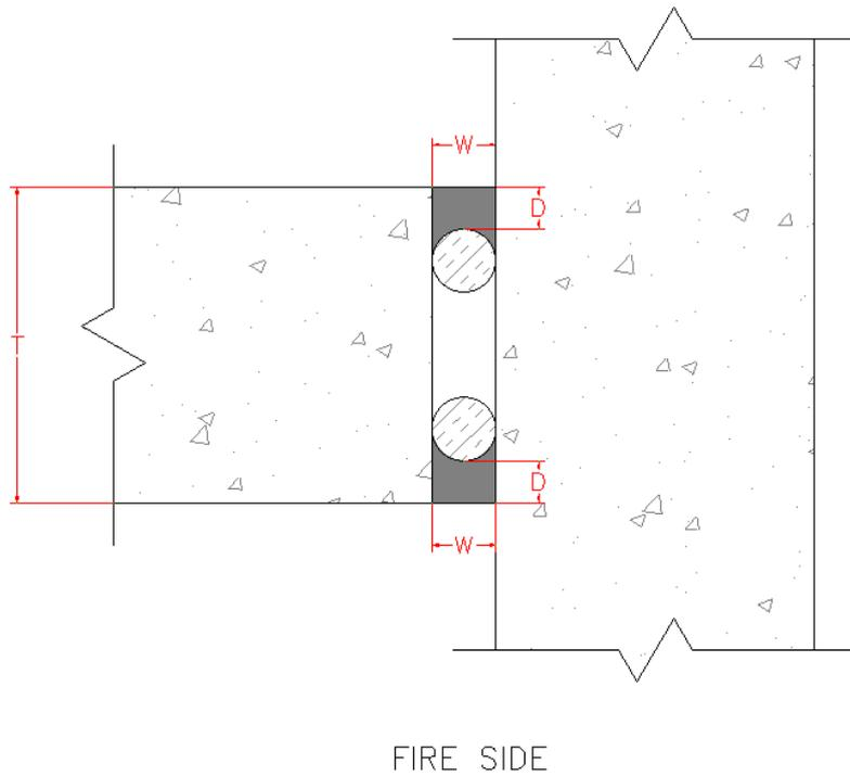
**Figure 5 – Typical sealant insulation**
