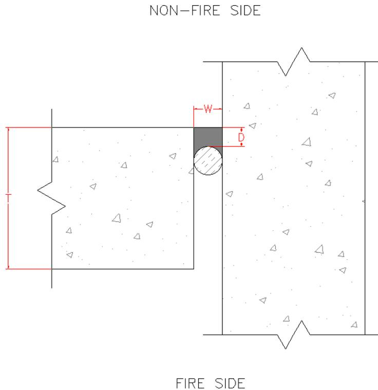
**Figure 6 – Typical sealant insulation**
