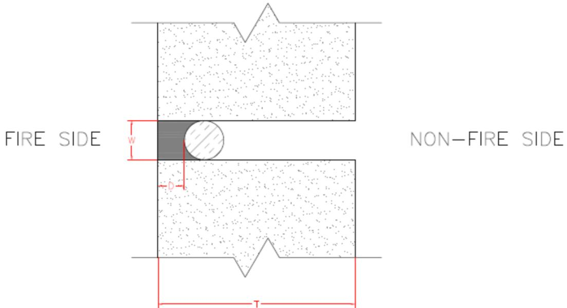
**Figure 8 – Typical sealant insulation**
