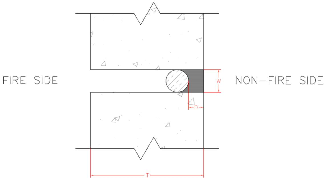
**Figure 2 – Typical sealant insulation**
