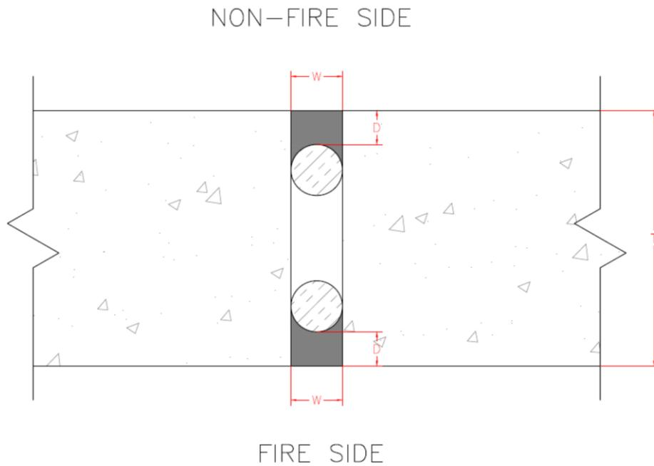
**Figure 3 – Typical sealant insulation**
