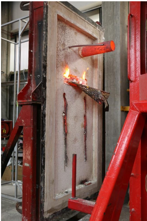
Photo 6: The Exposed Face of the Specimen Immediately After Testing
