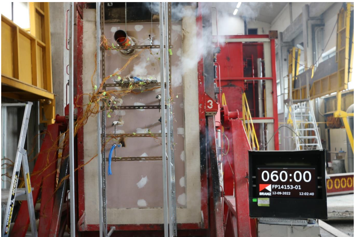
Photo 4: The Unexposed Face of the Specimen After a Duration of 75 Minutes
