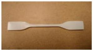
Fmax; This is the maximum tension (force) a sealant can absorb. It indicates the strength of a sealant. Fmax is expressed in N/mm<sup>2</sup>. Often Fmax (maximal strength) is written, but actually
